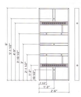
The multi-purpose panel can be used to form pilasters, corners, columns, bridge abutments and connections to existing walls. The panels have multi-adjustment profiles for mounting column clamps or ties.
